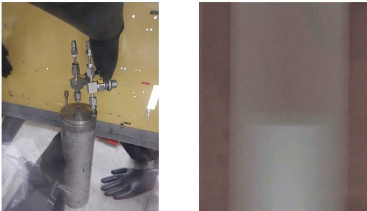
Figure 3: (left) NaK getter stored in the VNS-1 glovebox, (right) radiography of the NaK getter showing a sharp edge between the liquid and the gas indicating the absence of (NaK) oxides
