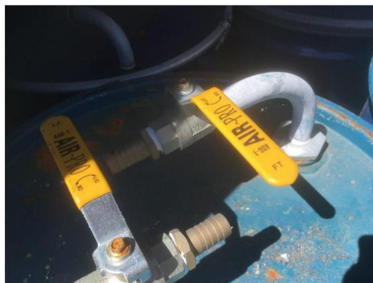
Figure 2: An example of the double valved lids used on the waste drums for the experimental drums
