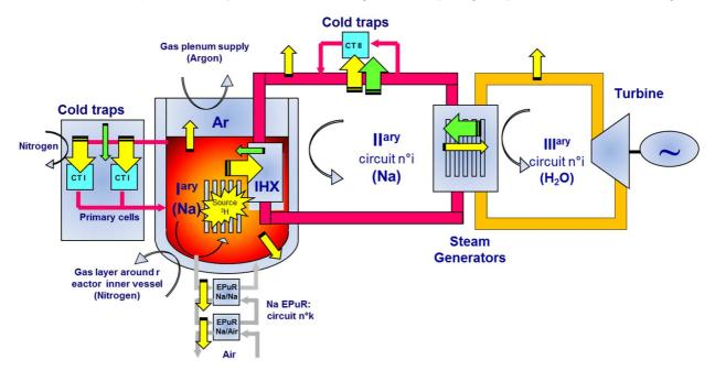
Figure 1 : Main tritium and hydrogen transfers in a SFR
