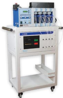
Figure 8: The WILMA online tritium monitor intended for use in drum sampling
